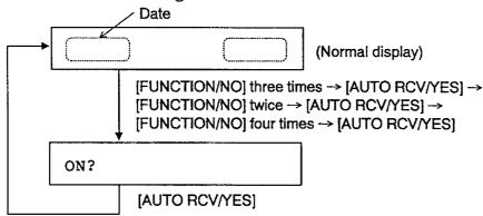
Then, set the receive mode to the "FAX" (Fax only) by pressing the [AUTO RCV/YES] button successively. Each press of this button changes the display as follows.
